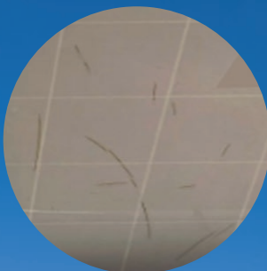
Widespread backsheet cracking PVDF
