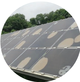
Glass/encapsulant delamination 8 years West India
