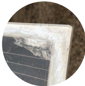
Delamination 9 years SW USA
