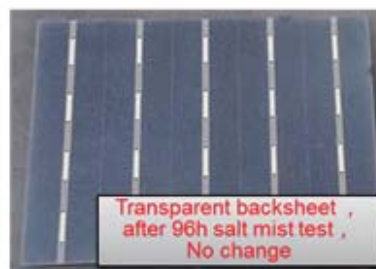
Figure 6. Anti-saline alkali comparison of transparent backsheet and glass
